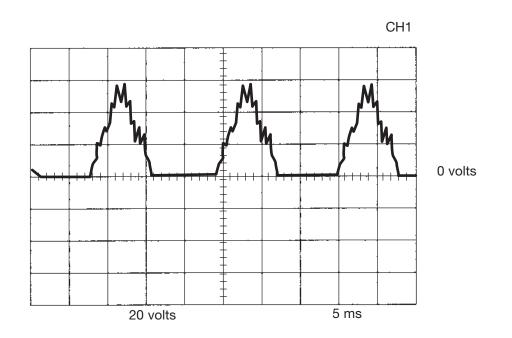
This is NOT the typical CV output voltage waveform. One output diode is not functioning. Note the "gap" in the waveform. One output diode was disconnected to simulate an open or nonfunctioning output diode. Each vertical division represents 20 volts and each horizontal division represents 5 milliseconds in time.
